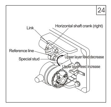
3.4 Adjust the upper feed mechanism (Fig. 23)
